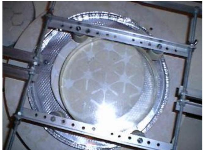
They seem to have done well however. Members watched while the grinding continued and the glass got clearer. For the final part of this stage, we used polishing rouge on the felt pads rather than the 9 micron grit.
