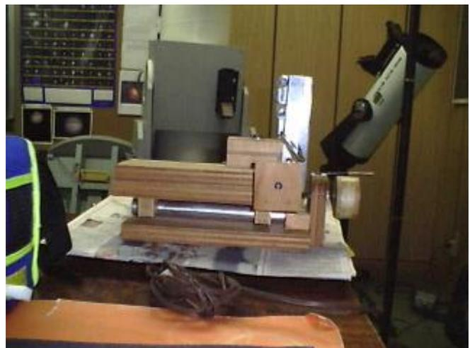
The larger shiny object holds a light which shines through a very narrow slit between two razor blades (seen taped at the top).
