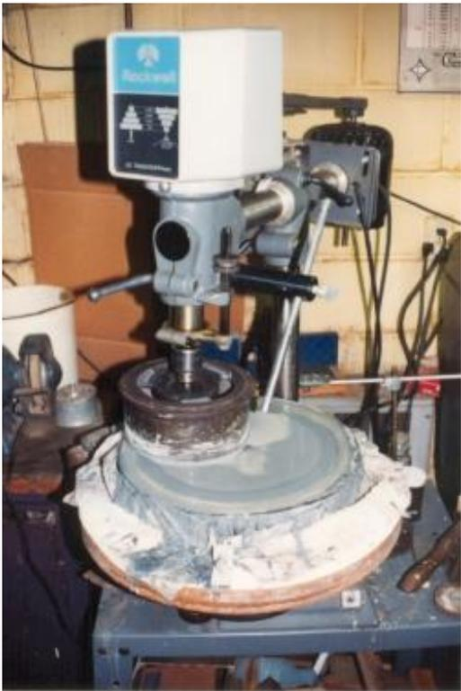
Those pathetic frozen pizzas have the perfect sized pans for making sure that the slurry formed by the grit and water would stay contained. While cleaning the turntable is not difficult, it could get messy if we did not constantly make sure the slurry was contained.
