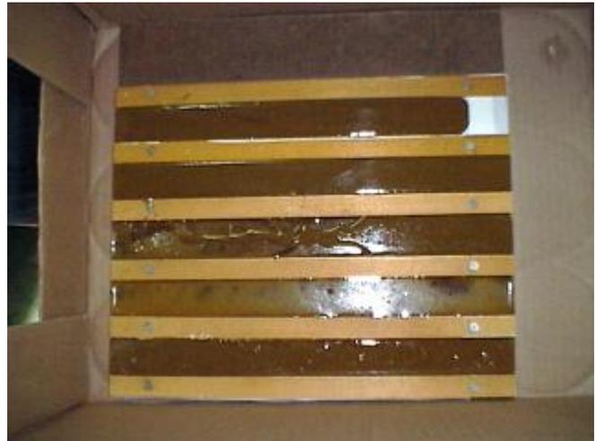
The concrete base of the tool was now covered with a thin layer of pitch. This helped make sure that no particles of concrete would come loose and scratch the mirror. It also provided the base that the squares of pitch would stick to.
