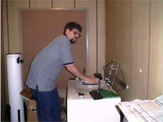
The Foucault test is one of many different tests designed to test the focal length, smoothness, and accuracy of the surface figure of a mirror (most of the other tests are just elaborations of this basic set-up). A good description is given in Texereau's classic *How to Make a Telescope*, copyright Interscience Publishers, Inc. 1957. Newer editions are available, but the basic design has not changed.
