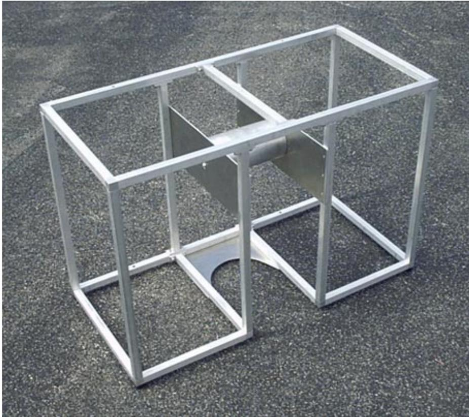
After a few hours of cutting aluminum tube lengths and pressing the fittings into them, the basic frame took shape. Then we added two 1/8" aluminum sheet plates to hold the altitude bearing, and since one section of the frame has to be left out so that the frame can be moved in altitude when on the pier, more 1/8" aluminum sheet was used as a gusset in the back to keep the two sides from sagging towards each other.
