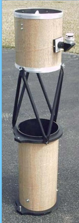
The secondary cage was made from a 12 1/4" piece of 10" ID Sonotube. (Sonotube for the whole project was donated by J&K Supply of Lafayette.) This section was made almost entirely by Jim Sattler.
