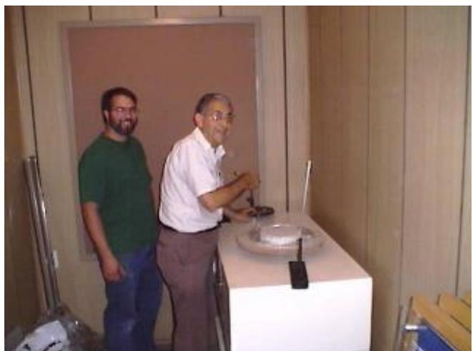
object to turn a bit at the end of each stroke. The relatively crude construction of the alligator also insures that the rotation of the upper object is not too consistent, which could introduce regular errors in the shape of the mirror due to the cyclic nature of the action. Randomness causes any errors to be distributed around the entire surface of the mirror and average out so a reasonably spherical shape will be formed.
