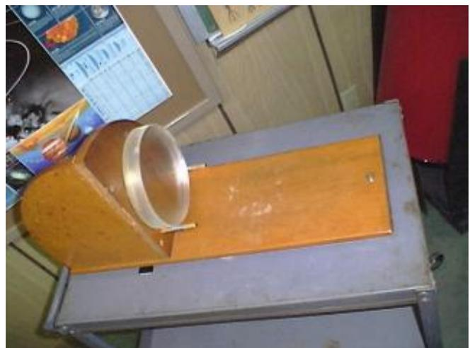
Usage of the Foucault tester started in February. While the mirror was not really ready for testing, it was satisfying to test the mirror and see a dim pattern in the expected form. The room is darkened since the image is quite dim. (Remember, it has not been aluminized yet!) We had to make sure to warn both Jim and John before the flash went off, since eyes need to be adapted to low light levels to see the reflected light.
