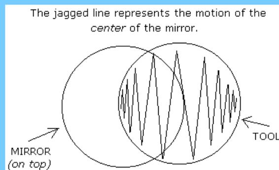
Here the action is concentrated when the mirror is near the edge of the tool. In that situation, the weight of the mirror is resting on its center, so the mirror gets worn away more there. Both the mirror and tool are rotated frequently so the action is evenly distributed (in terms of the angle, *but not the distance* from the center). Strokes that hollow out the center rather than lowering ("reducing") the edge seem to be more commonly used, probably because of the danger of
